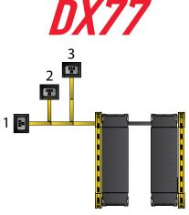
Manufacture provided 60" (standard length) air and hydraulic hoses allow three ergonomic, recommended power console placement options.
